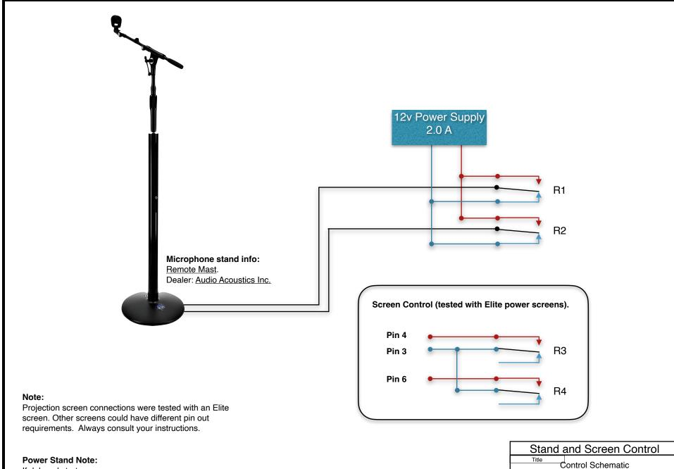
If delayed start, use 1000  $\mu\text{F}$  capacitor on PS output.
