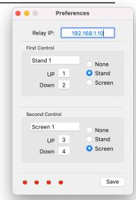
The 3 LEDs show current status of relay. Red is off and green is on. If the stand is backwards (up is down and down is up) just invert the two relay numbers and try again.
